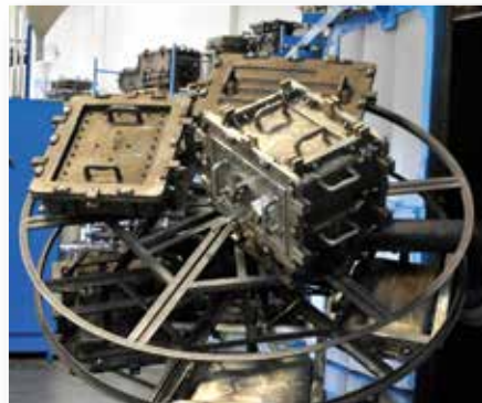
Pictured: Molds rotating during production.
