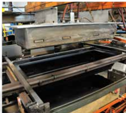
Pictured: Vacuum mold for keyboard case.
